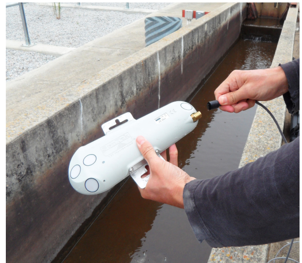
The SonTek-IQ is a multi-beam acoustic flow meter with five 3.0 MHz transducers. Redundant water level data are recorded from the vertical beam and pressure sensor. Data download and communication are available via RS232, Modbus or SDI-12. Flow rates and total water volumes are computed internally based upon a user supplied survey of the channel shape and instrument location.
